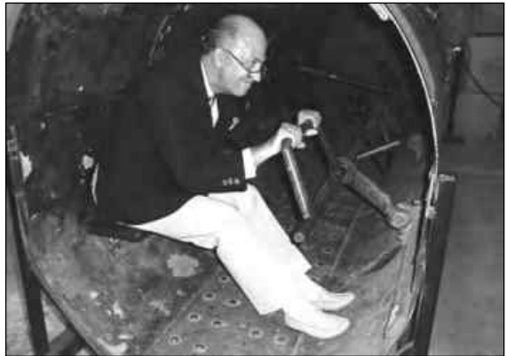
Serge rotates the propulsion crankshaft of the "Hunley" replica that was built for the TV film of the same name.
